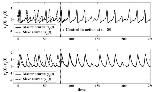
Fig. 6. Time responses of states for master and slave FN neurons
